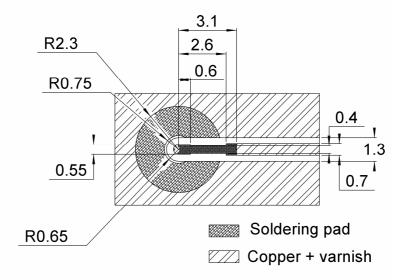
Substrate: RO4350 thickness 0.254mm, with copper layer 35µm on both sides: Add vias between both sides along upper ground plane according to engineering practise
